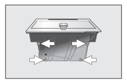
■ Push the appliance all the way back into the cabinet and center it. If necessary level the unit with the four height adjustable feet.
